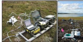
Fig. 2. Multicomponent FTIR Gas analyzer combined to 4 automated dark chambers. The FTIR, computer, gas flow controller, and pump system were installed on a ladder to facilitate transport.
